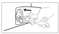
11. Replace the emergency emptying cap into the filter cover and fix it firmly.
